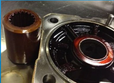
Varnish on the housing cover of the hydraulic pump
